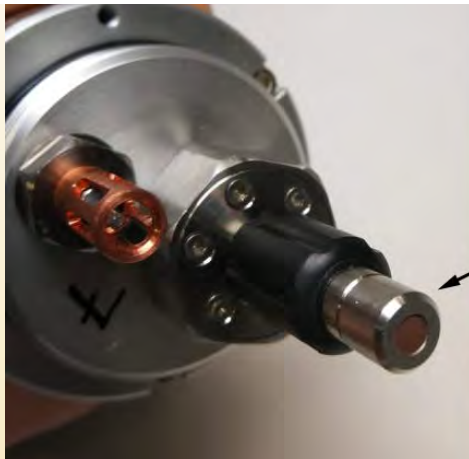
Screw-able cap with sensing material (pH or O 2 )
