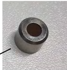
Screw-able cap with sensing material (pH or O 2 )
