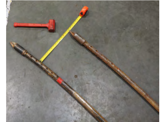
Post test pipe geometry within tolerance
