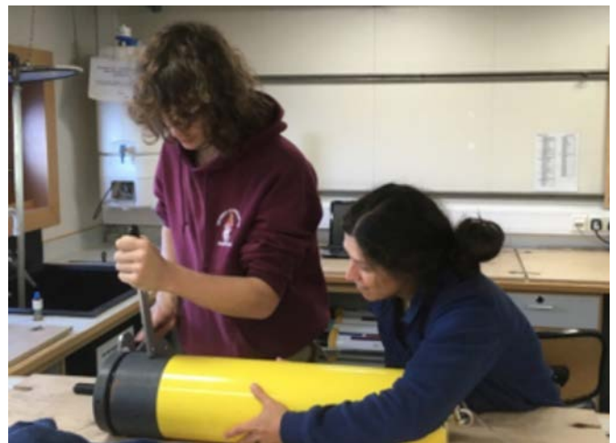
Above: Gaye Bayrakci and Dan Ellis opening up the acoustic recorder to recover the data. The acoustic recorder was used to record the seismic sources within the water column, as well as the methane bubbles.
