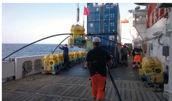
Above: deployment of an Ocean Bottom Electro-Magnetic (OBEM) receiver
